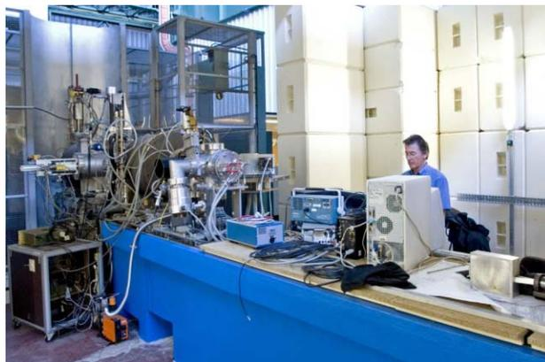
Figure 2: View of the source and the LEBT at Saclay. A part of the LEBT is located on the RFQ concrete support.
