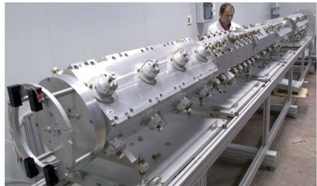
Figure 5: Six-meter long cold model of the RFQ used to develop the tuning process of the IPHI cavity.
