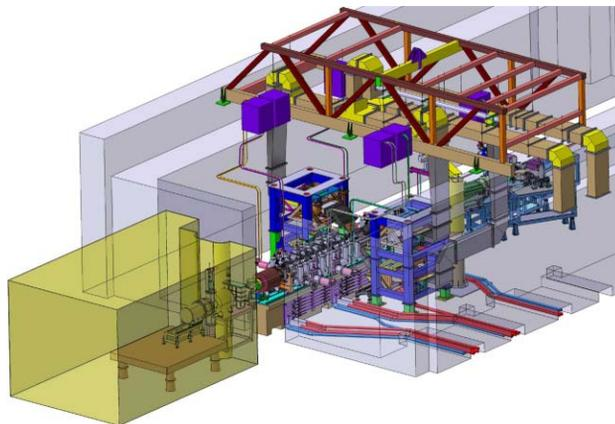
Figure 1: 3D view representing the final arrangement of the IPHI injector.
