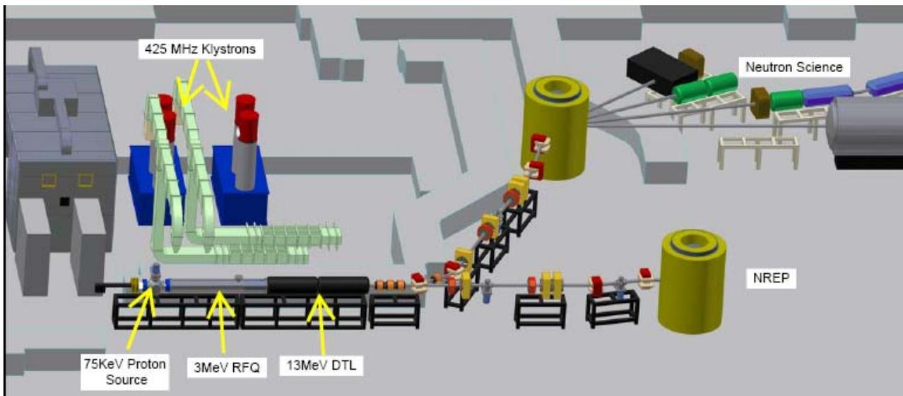
Figure 1: Layout of the Phase 4 LENS project with a 13 MeV, 100 mA proton accelerator shown installed. The 3 MeV RFQ is 3 meters long. The 13 MeV Phase 2 version will require 3 klystrons and a conceptual 22 MeV Linac would require 5 klystrons.
