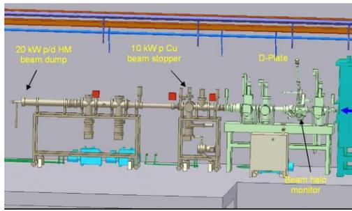
Figure 4: The D-plate and the two beam dumps as they are to be installed downstream of the PSM.
