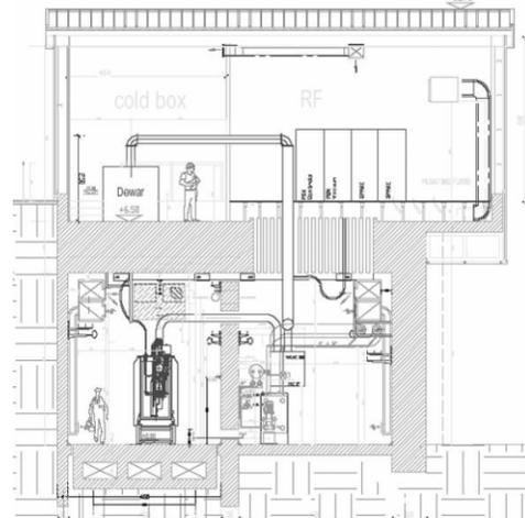
Figure 5: Cross section of the building including the beam and service corridors and the RF and cryogenics halls.
