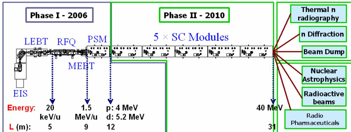
Figure 1: Schematic layout of SARAF. The architecture of the accelerator is displayed, including the length and ion energy at each stage. The division to Phase I and Phase II (including anticipated applications) is shown.
