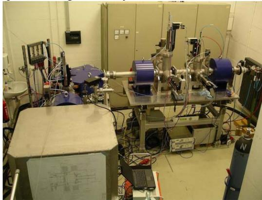
Figure 2: The ECR ion source (inside an HV cage) and the LEBT at Accel premises.
