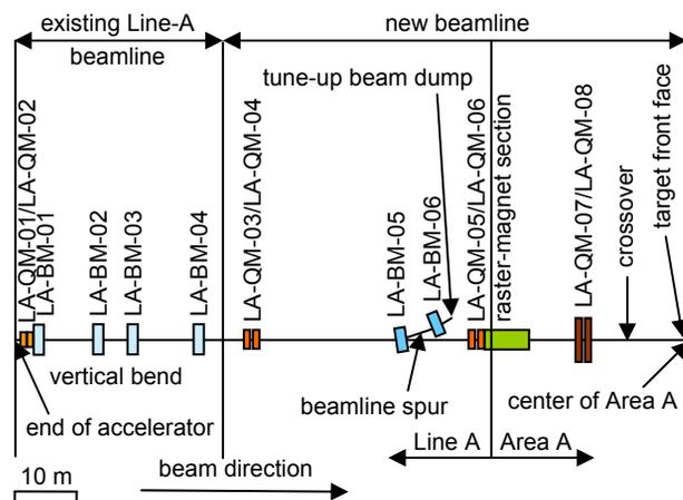
Figure 1: Sketch of beamline from end of LANSCE accelerator to MTS-target front face, and of beamline spur to tune-up beam dump.
