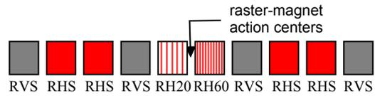
Figure 4: Likely raster-magnet-section configuration, with two pairs of slow horizontal magnets (RHS), two pairs of slow vertical magnets (RVS), a 20-kHz magnet (RH20), and a 60-kHz magnet (RH60).
