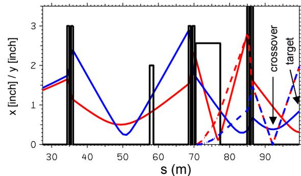
Figure 3: Horizontal (red) and vertical (blue) 7-rms beam envelopes (solid lines) and beam-centroid excursions (dashed lines) in new beamline. Element positions and apertures are indicated in black.
