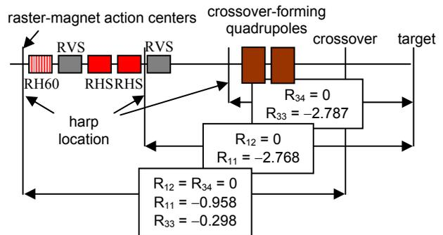
Figure 5: Sketch of beamline from raster-magnet action centers to target, showing locations of harps used to determine beam sizes at crossover and target. Relevant transfer-matrix elements are given.
