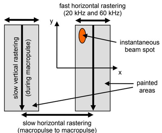
Figure 2: Painted areas at target, and instantaneous beam spot. Painting involves slow horizontal and vertical rastering and fast horizontal rastering.
