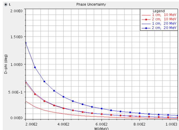
Figure 3: Cavity phase scaling error vs. beam energy, arising from cavity position uncertainty. Cases are shown for 10 and 20 MeV beam energy changes due to cavity failure. .
