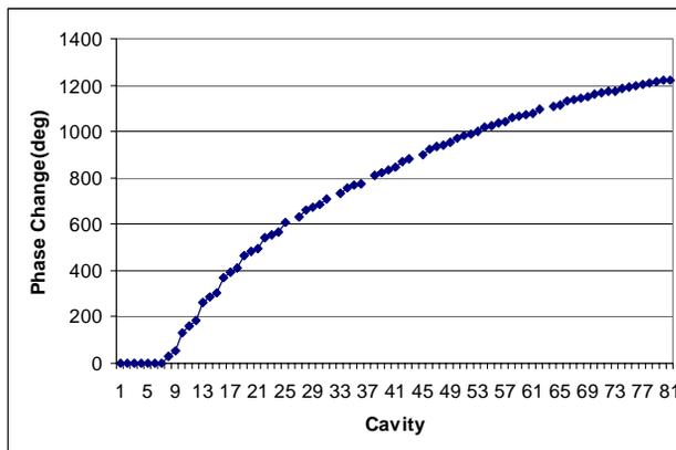
Figure 5: The predicted cavity phase setpoint change resulting from turning off cavity 7. The last cavity phase setpoint was checked with a phase scan and found to be within 1 degree of this prediction.
