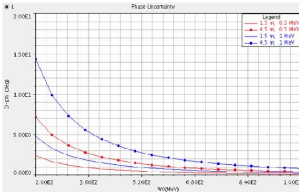
Figure 4: Cavity phase scaling error vs. beam energy, due to beam energy gain uncertainty. Cases are shown for 0.5 and 1 MeV beam energy change uncertainty and for cavity separations of 1.5 and 4.5 m.
