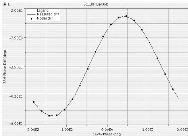
Figure 2: Typical phase scan result showing the measured beam phase difference vs. the cavity phase. Lines are measurements and dots are model predictions with matched values for field, RF phase offset to the beam, and input beam energy.
