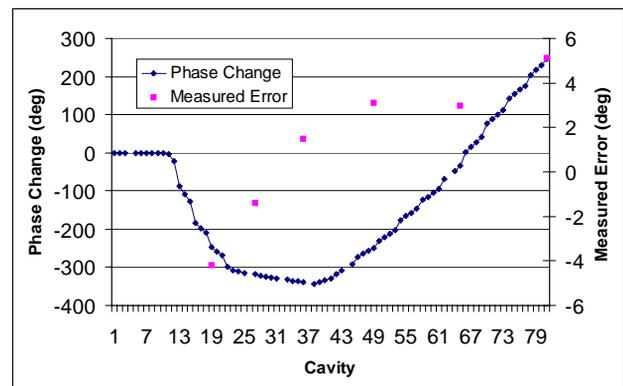
Figure 6: The predicted cavity phase setpoint change resulting from turning on cavity 10 and reducing 11 additional downstream cavity amplitudes. Some phase setpoint errors (checked by the phase scan) are indicated.
