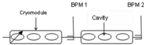
Figure 1: Schematic of the phase scan technique for determining the beam phase relative to the RF, where the BPMs provide an absolute beam phase measurement.
