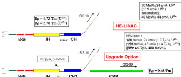
Fig. 3: Long-term LINAC-option for high intensity heavy ion beams for the FAIR accelerator facility.
