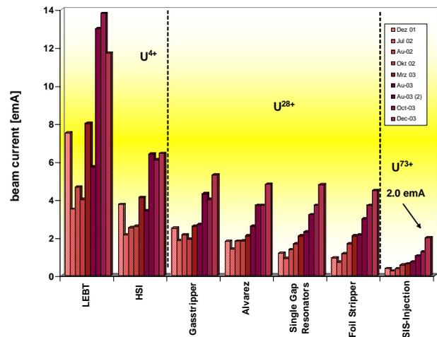
Fig. 2: Improvement of the UNILAC-Uranium beam intensities [2].
