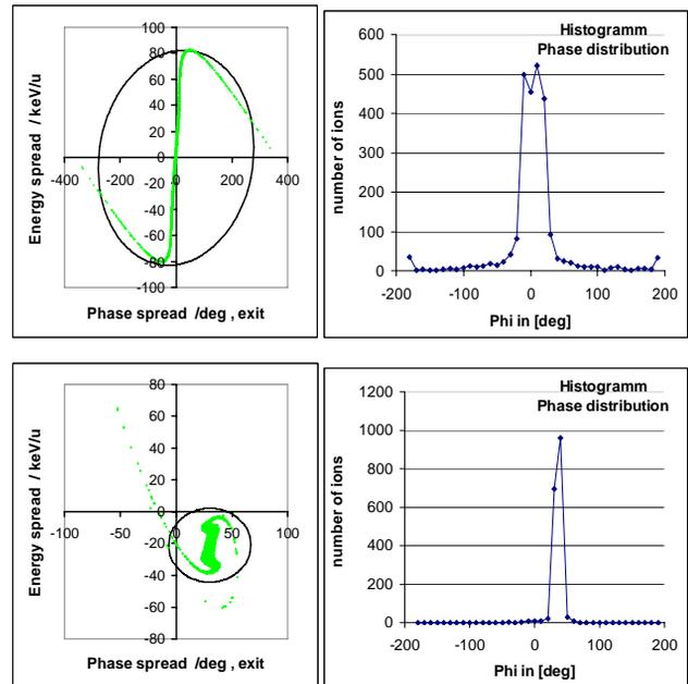
Figure 2: Longitudinal phase space of the beam bunched by the DDB at the entrance of the IH-structure (upper panels) and at the exit of the IH-structure.
