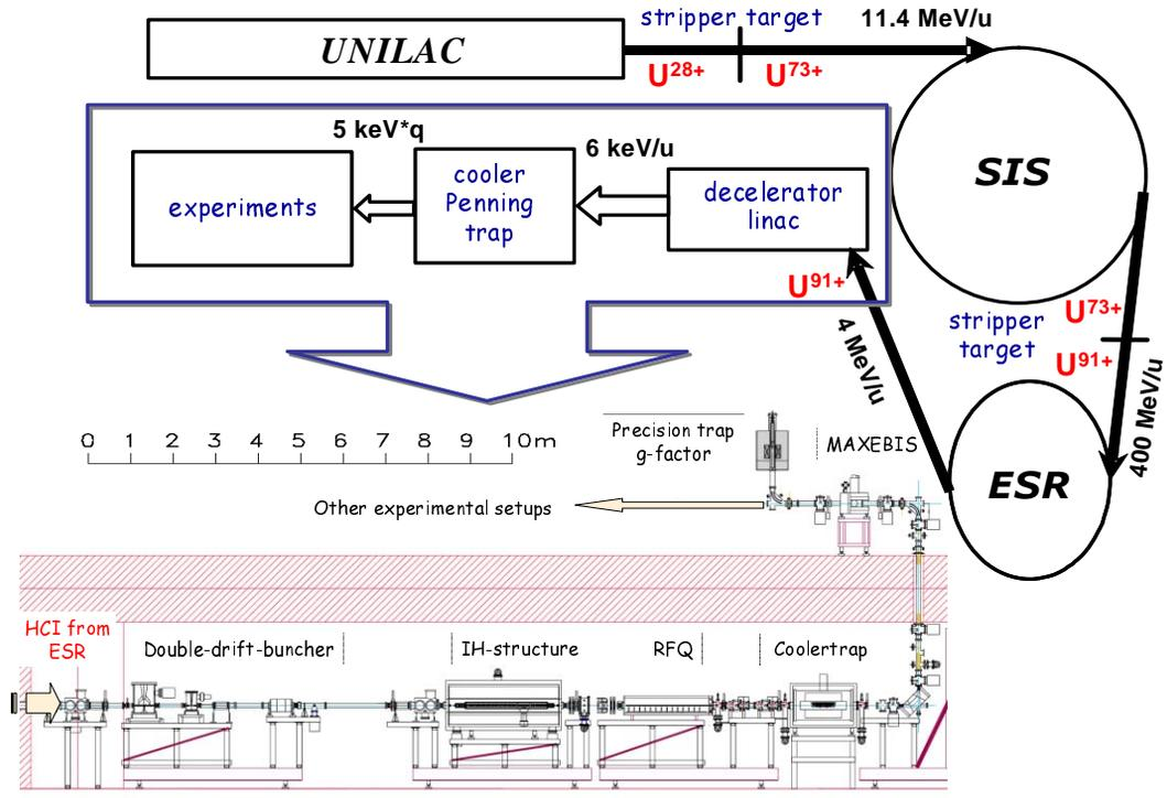
Figure 1: Schematic of the GSI accelerator chain and the HITRAP LINAC
