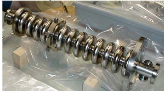
Figure 2: FNAL CKM 13-cell deflecting mode cavity.
