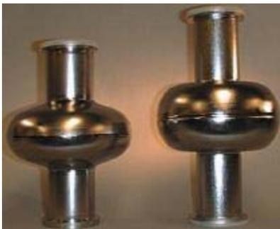
Figure 1: Single-cell from TESLA cavity (left) and a corresponding cell from a re-entrant cavity (right) fabricated by the Cornell University SRF group [6].
