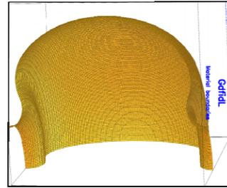
Figure 3: GdfidL mesh consisting of  $1.45 \times 10^6$  elements for a one quarter section of a single RE cell. Each mesh element is separated from its neighbour by 1mm.
