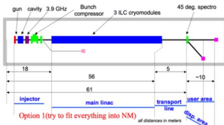
Figure 6: Current plan of ILC test accelerator in NM.
