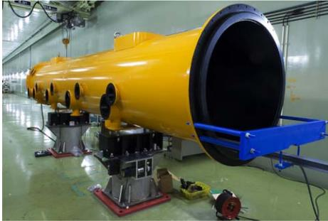
Figure 8: Half size cryostat vessels to be used in STF phase 1 accelerator are delivered to STF.
