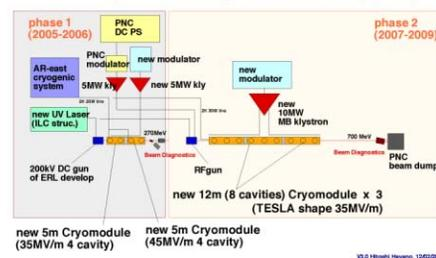
Figure 7: STF phase 1 and phase 2 plans.
