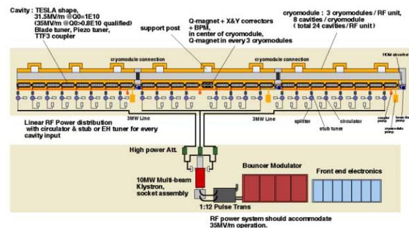
Figure 2: RF unit configuration of ILC main linac.
