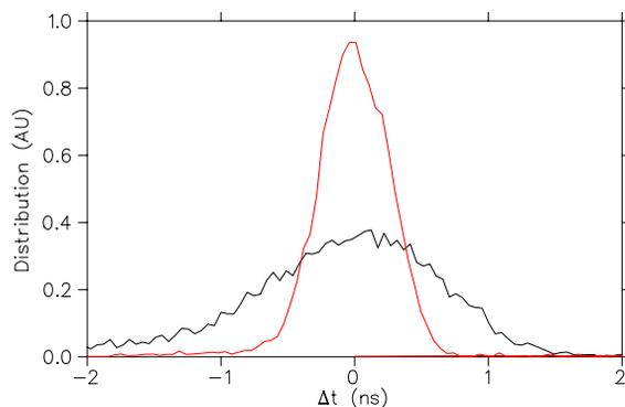
Figure 7: Time spectra recorded at a silicon detector with and without cavity 19 used as a buncher. Cavity 1-8 are ‘on’ producing a beam energy of 3.7 MeV/u.
