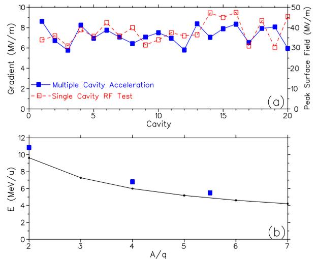
Figure 5: (a) Average cavity gradients for the three  $A/q$  values and for 7 W cavity power. Results are inferred from the step energy gain per cavity during acceleration. Also shown are gradients from initial single cavity characterizations. (b) Final energies for the three cases compared to expected final energies assuming the design gradient of 6 MV/m.
