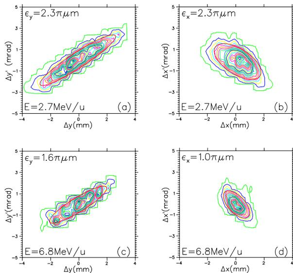
Figure 6: Shown are the vertical (left) and horizontal (right) transverse emittances measured downstream of the linac for  $4\text{He}^{1+}$  at two different energies, 2.7 MeV/u and 6.8 MeV/u.
