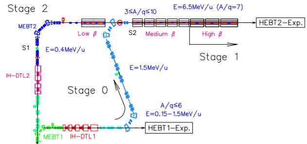
Figure 1: Stages 0, 1 and 2 for the ISAC-II upgrade.
