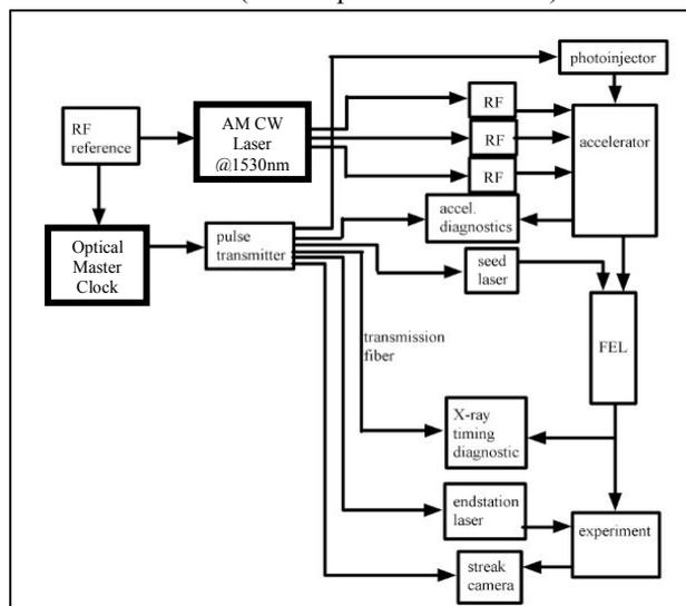
Figure 5: Schematic representation of the FERMI@elettra timing and synchronization system.
