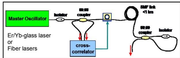
Figure 3: Fiber optics link stabilization “a la MIT”.
