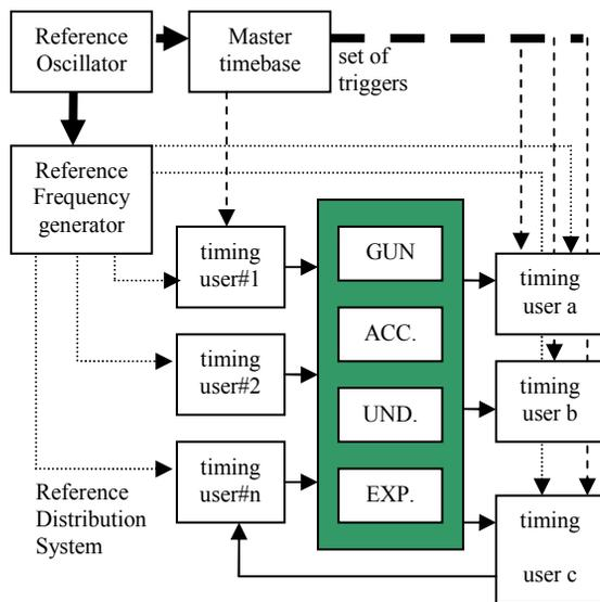
Figure 1: Schematic representation of a T&S system.
