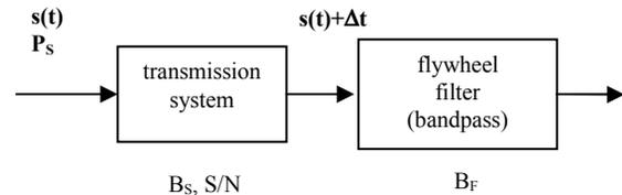
Figure 2: Block diagram of a transmission system plus band pass receiver filter.
