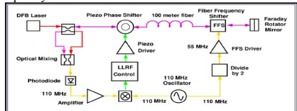
Figure 4: LBNL fiber optic stabilized link.
