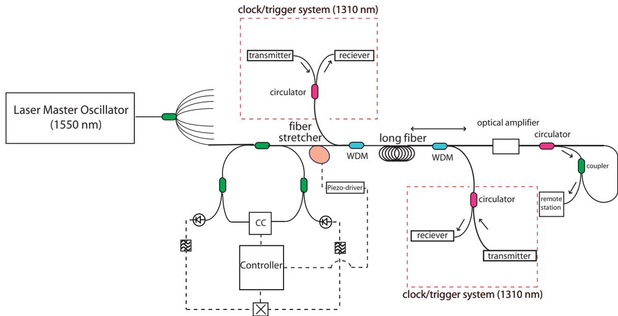
Figure 2: Schematic of the integrated synchronization and clock/trigger distribution system (CC - cross correlator, WDM - wavelength division multiplexer, transmitter - 1310 nm laser with amplitude modulator)
