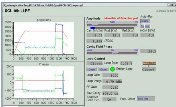
Figure 5: This beam loading response of the FCM on a high-beta cavity demonstrates the very wide control dynamic range that the FCM has.
