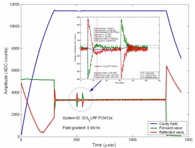
Figure 3: The FCM step response measured on the medium-beta cavity SCL-12a indicates that the feedback has a closed-loop control bandwidth greater than 50 kHz.
