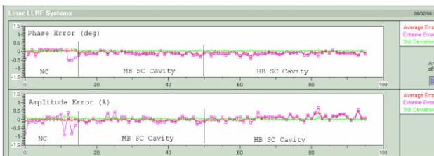
Figure 6: Linac-wise system performance of rf control measured in a recent beam run. The beam current is 20 mA, and the beam pulse length is 200 us.
