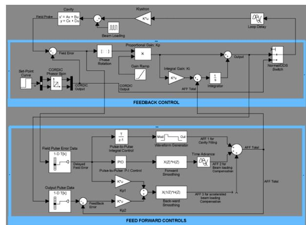
Figure 1: The combined feedback and feed forward control scheme is used in the field control module in SNS Linac.
