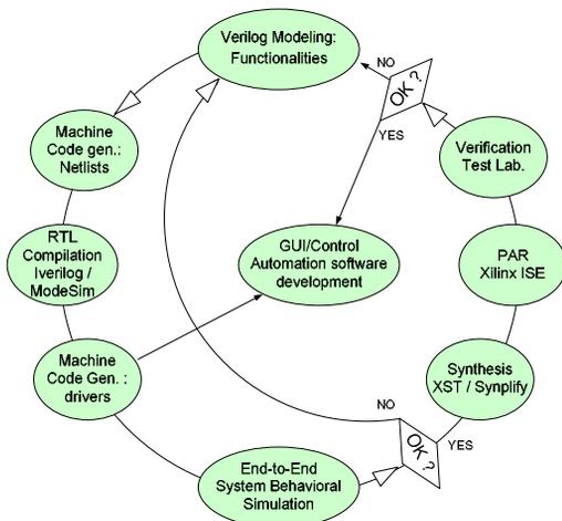
Figure 2: The automated development and co-simulation process for the FCM.
