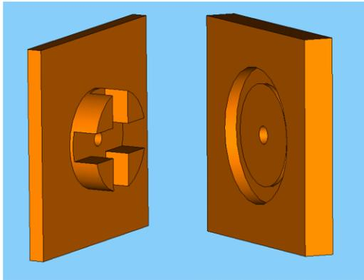
Figure 2: The MWS models of the SNS RFQ's entrance plate (left) and exit plate (right)
