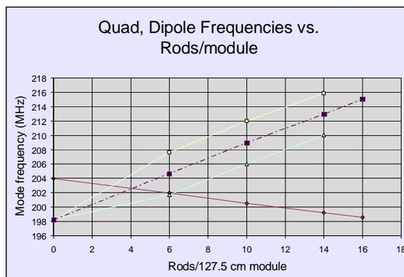
Figure 6: MWS simulations of quadrupole and dipole frequencies as a function of the number of  $\pi$ -mode rods per 127.5-cm long module.
