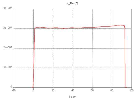
Figure 4: Simulated electric field flatness of the quadrupole model along the MWS RFQ model with as-built SNS RFQ dimensions and final tuner positions.
