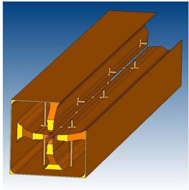
Figure 1: A sectional view the 3-D simulation model of the SNS RFQ by CST Microwave Studio. Radial matcher,  $\pi$ -mode stabilizers (rods) and exit cut-back are included in the model.
