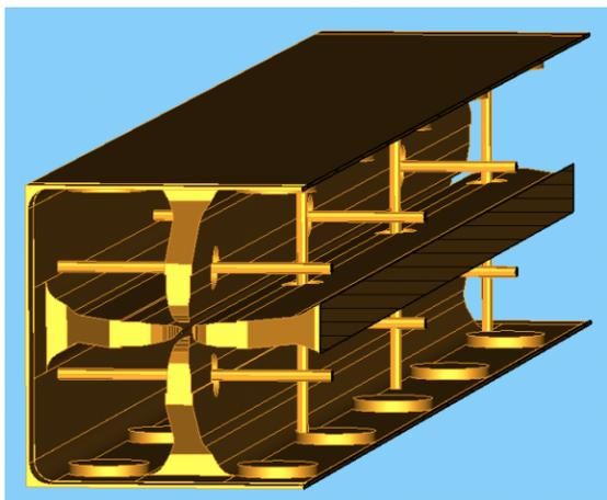
Figure 5: The MWS model shows the layout of the  $\pi$ -mode rods and tuners for the SNS RFQ.
