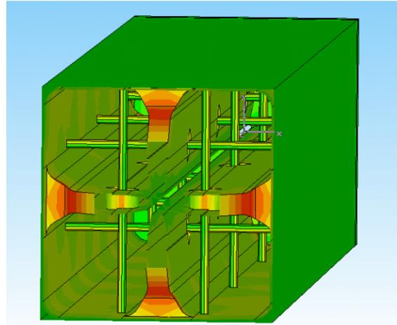
Figure 3: RF power dissipation distributions on the SNS RFQ structures. Hot spots (red color) or high power dissipation areas are located at the cut-backs of the vanes.
