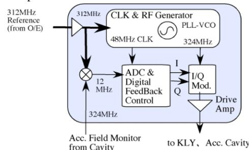
Figure 5: Feedback control system. Refer to [4] for the detail.
