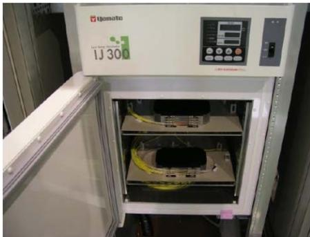
Figure 2: The 1x17 optical coupler in an oven.
