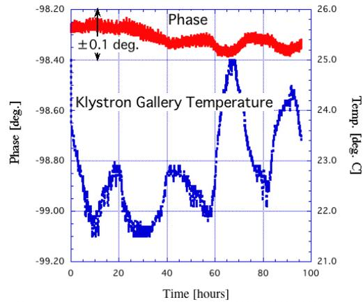
Figure 8: Result of the measurement of the phase stability of the RF reference.
