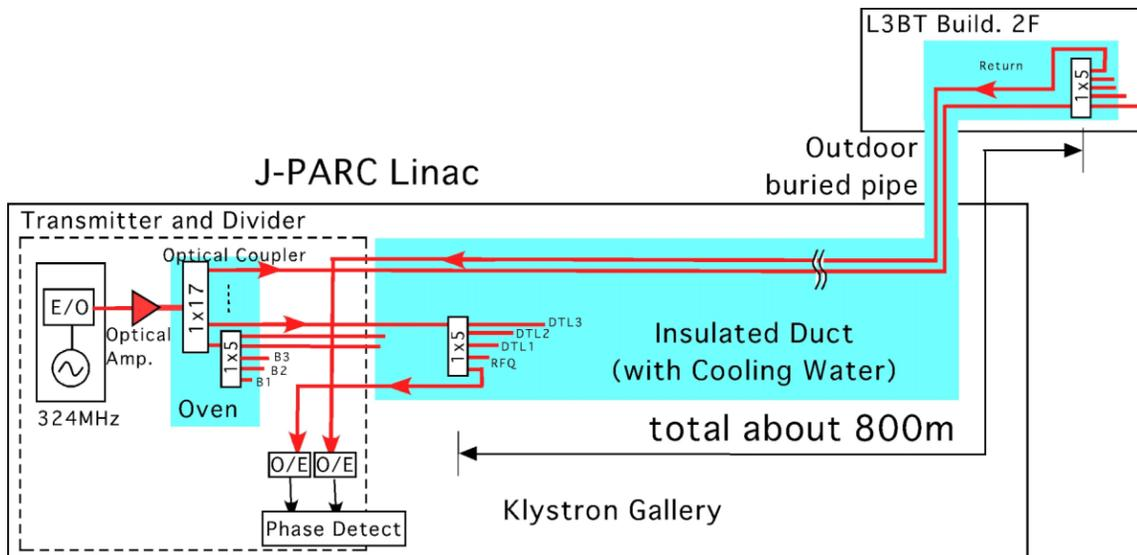
Figure 7: Measurement of the phase stability of the RF reference.
