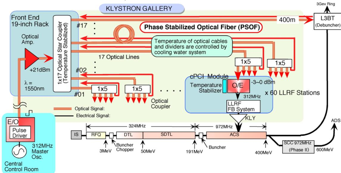
Figure 1: Block diagram of the RF reference distribution system.
