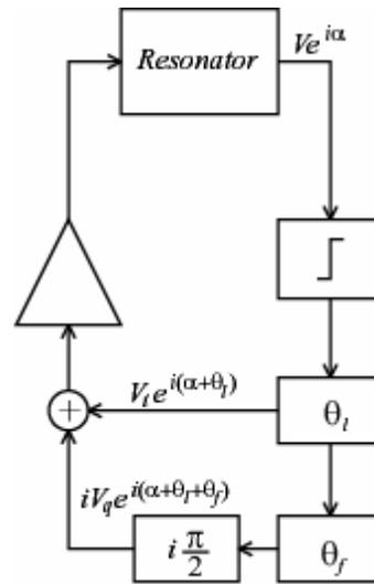
Figure 1: Self-excited system with phase locking.
