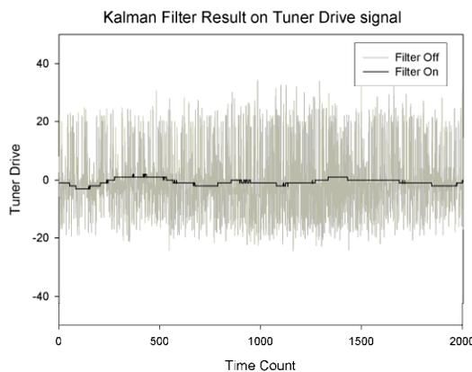
Figure 3: Tuner drive signal with/without filter.
