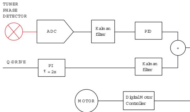
Figure 2: Placement of Kalman filters in tuner control loop.
