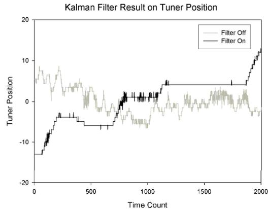
Figure 4: Tuner position with/without filter.
