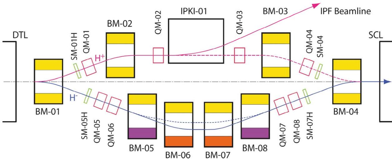
Figure 1: Transition Region of the LANSCE Linac. The bend magnets in the  $H^-$  branch are served by two power supplies, each, adding their currents for BM-06 and -07 and subtracting them from each other for BM-05 and -08.
