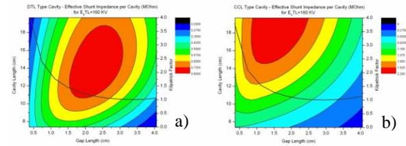
Figure 4: Effective shunt impedance ( $M\Omega$ ) and the Kilpatrick curve for a DTL-type cavity (a) and a CCL-type cavity (b).
