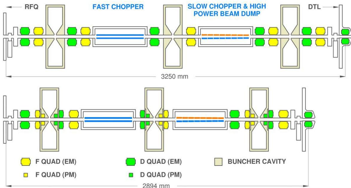
Figure 1: Two possible MEBT configurations showing a reduction in length using compact components.
