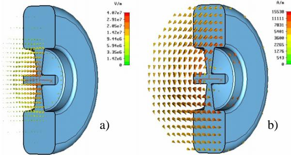
Figure 2: Microwave Studio 3D model of a DTL type cavity: a) Electric Field Vector, b) Magnetic Field Vector.
