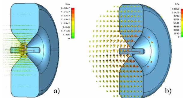
Figure 3: Microwave Studio 3D model of a CCL type cavity: a) Electric Field Vector, b) Magnetic Field Vector.
