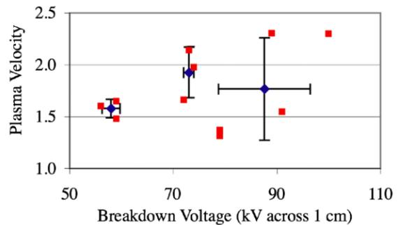
Figure 4: Plasma velocity (cm/ $\mu$ s) versus CDU voltage.
