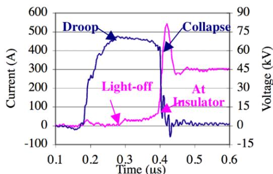
Figure 6: Current and voltage signals for 2.5 mm case.
