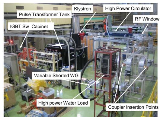
Figure 5: Picture of the STF rf test stand.
