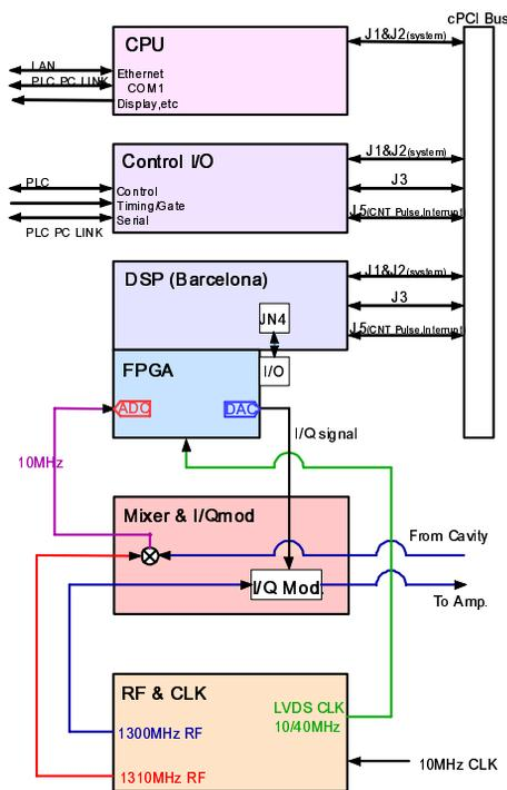
Figure 7: Block diagram of the digital LLRF control system for STF.
