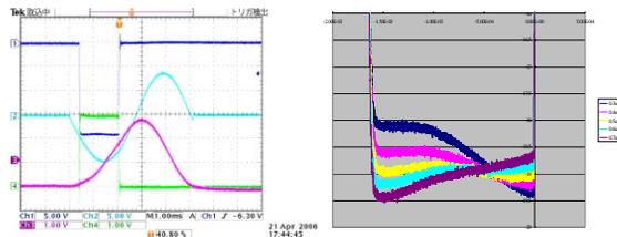
Figure 4: Left figure shows the pulse waveform (blue), bouncer voltage waveform (light blue) and bouncer current waveform (red). Right figure shows the variation of the flatness with the change of the timing of a bouncer trigger.
