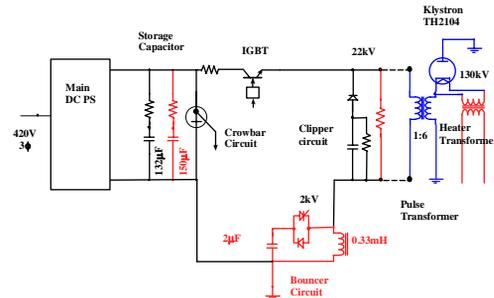
Figure 2: Block diagram of the revised modulator. Red parts are newly added and blue parts are modified.
