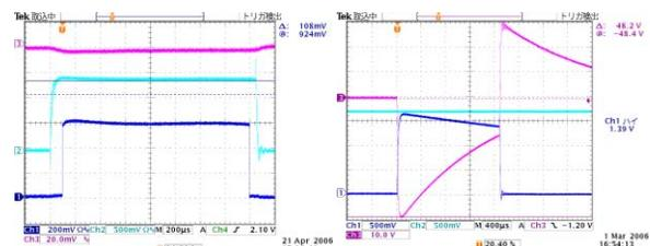
Figure 3: Current pulse waveforms with the bouncer circuit on (left blue) and off (right blue). Flatness was improved from 12% to  $\pm 0.4\%$  in this case.
