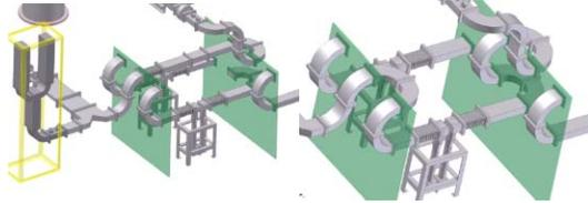
Figure 6: Examples of the waveguide system. Left shows the power distribution from the klystron to the water load. Right shows the power distribution for the coupler test.
