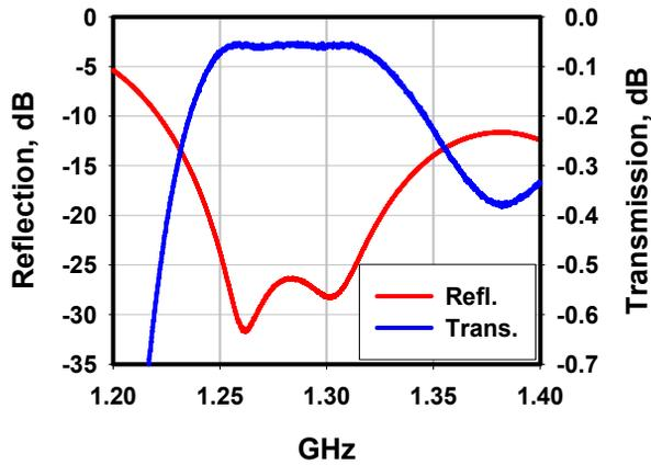
Figure 3: Measured passband of single coupler.
