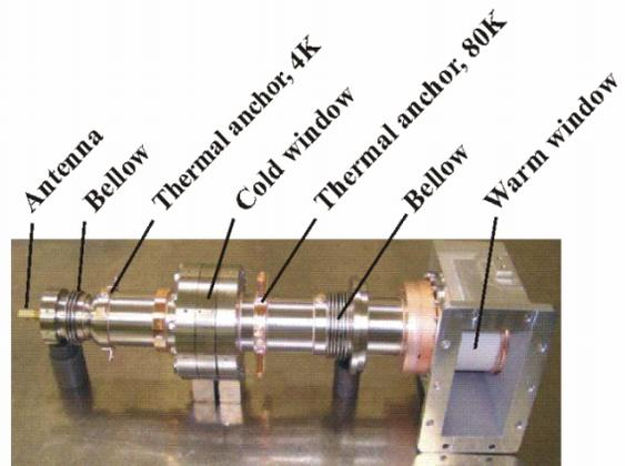
Figure 2: Assembled coupler.
