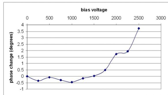
Figure 2: Phase shift at 468 MHz versus applied bias voltage in volts.
