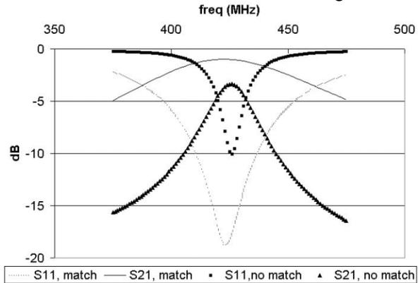
Figure 4: Simulated match performance with and without alumina match.
