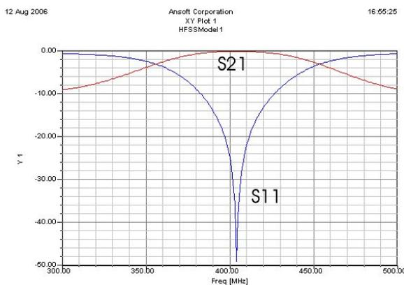
Figure 7: Simulated transmission for BST phase shifter (no DC bias).
