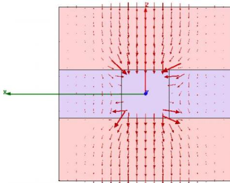
Figure 3: Higher Order TE mode in a Square TEM waveguide loaded with BST bars on top and bottom of the inner conductor.
