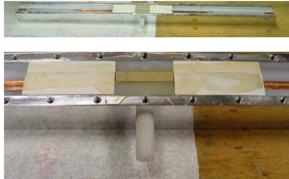
Figure 1: Prototype phase shifter showing BST bar (center) surrounded by two alumina matching sections with hole in center for DC feed.
