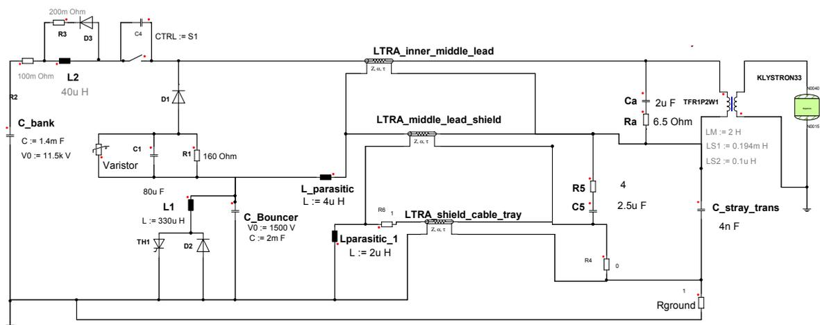
Figure 2: Simulation model of the modulator, pulse cable, adaptation network and klystron.
