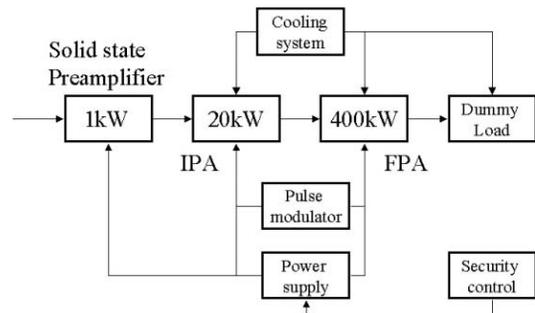
Figure 1: Schematic diagram of 400kW amplifier.
