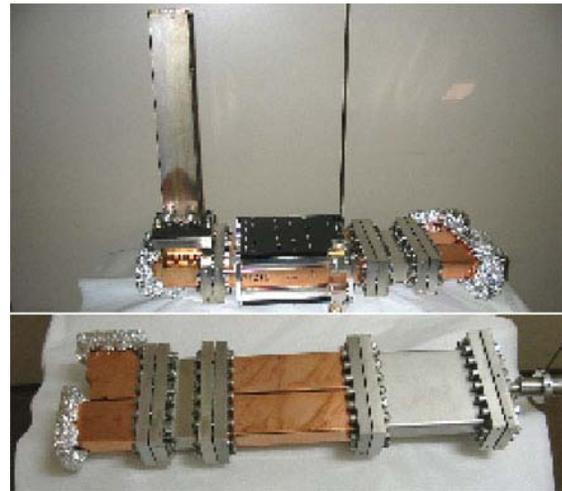
Figure 3: Factory tests of the 20 dB waveguide attenuator (up) and the  $2\pi$  phase-shifter (down).
