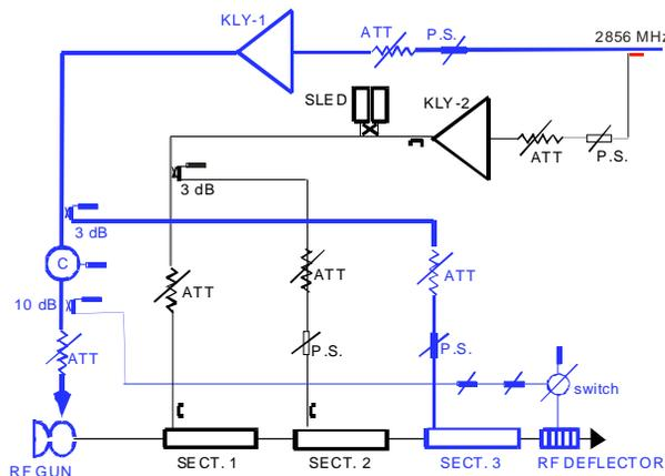
Figure 1: Layout of the SPARC RF system.
