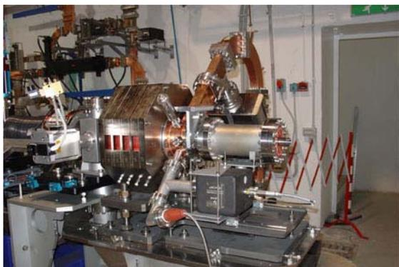
Figure 4: SPARC RF gun assembled at LNF.
