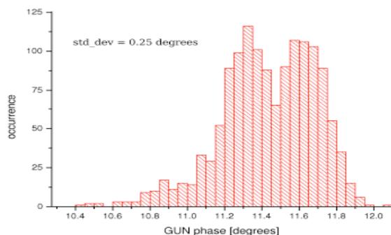
Figure 6: RF gun phase noise statistic distribution.
