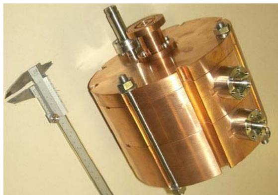
Figure 5: Two assembled deflector copper cells.
