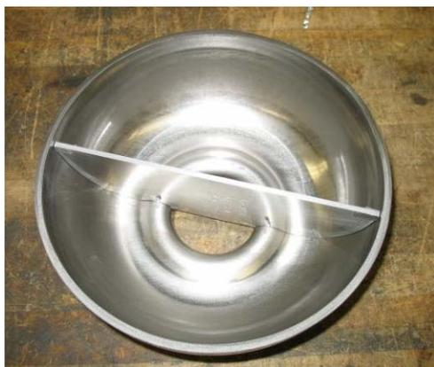
Figure 3: Reentrant half-cell with checking fixture.
