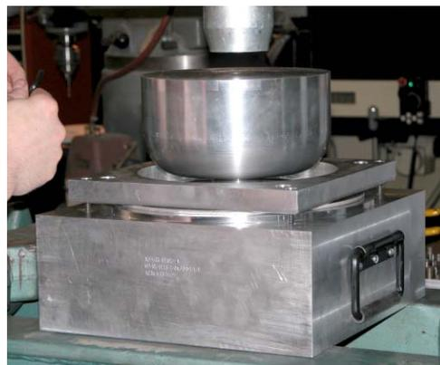
Figure 2: Deep drawing of non-reentrant half-cell with 75 tons.
