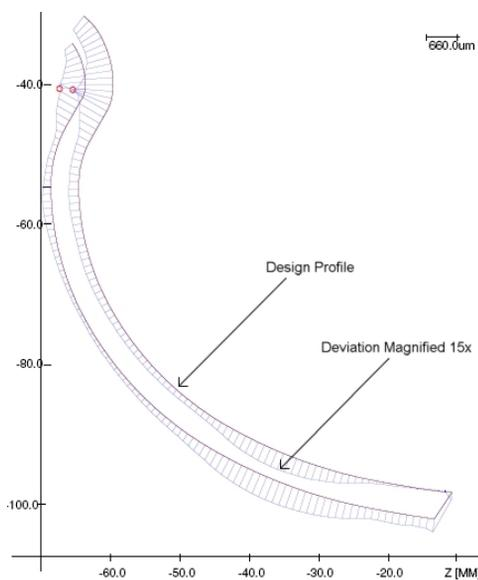
Figure 5: Coordinate measurement of reentrant half-cell after iris weld.
