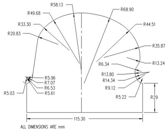
Figure 1: Mid-cell shape of fabricated half-reentrant cavity.
