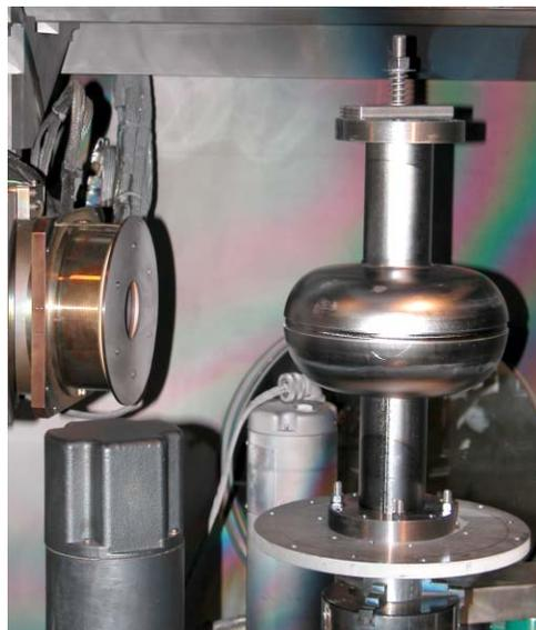
Figure 4: Full penetration e-beam weld of equator.
