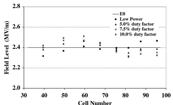
Figure 3: DTL2 Field Distribution versus Duty Factor after Coolant Passage Cleaning.
