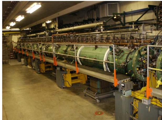
Figure 1: LANSCÉ Accelerator DTL2 with DTL1 in the background. The slug tuners can be seen mounted at their 45° angle between the drift tubes (top) and post couplers (side.)
