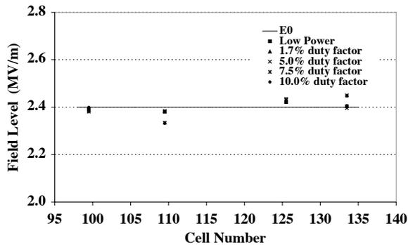
Figure 5: DTL3 Field Distribution versus duty factor after coolant passage cleaning.
