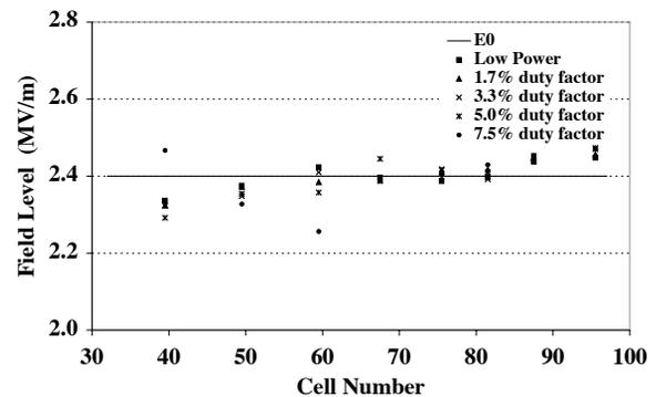
Figure 2: DTL2 Field Distribution versus Duty Factor before Coolant Passage Cleaning.
