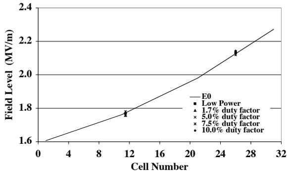
Figure 4: DTL1 Field Distribution versus duty factor after coolant passage cleaning.
