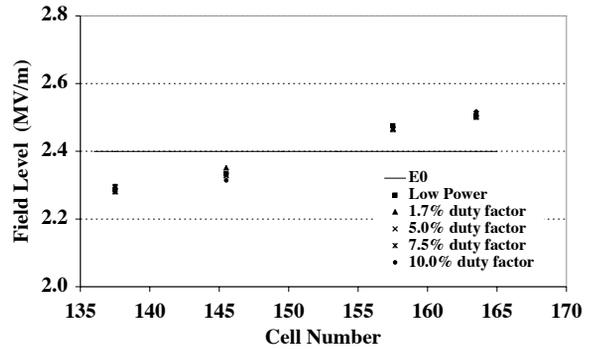
Figure 6: DTL4 Field Distribution versus duty factor after coolant passage cleaning.
