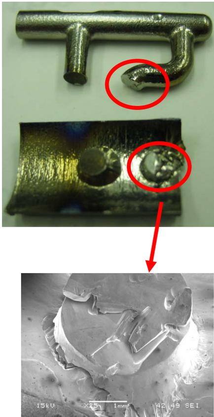
Figure 1: Fractured F-piece removed from Cavity 2 and SEM image of same. The break occurred on the right leg.
