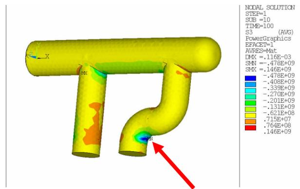
Figure 2: FEA stress analysis of fractured F-piece. The highlighted area indicates high compressive stress at the bend where the break occurred.
