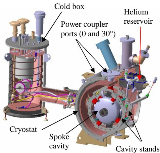
Figure 7: Inside view of the cryostat and cold box.
