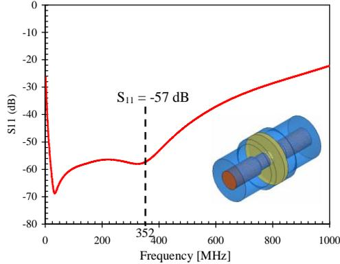
Figure 6: Calculated window reflection parameter.
