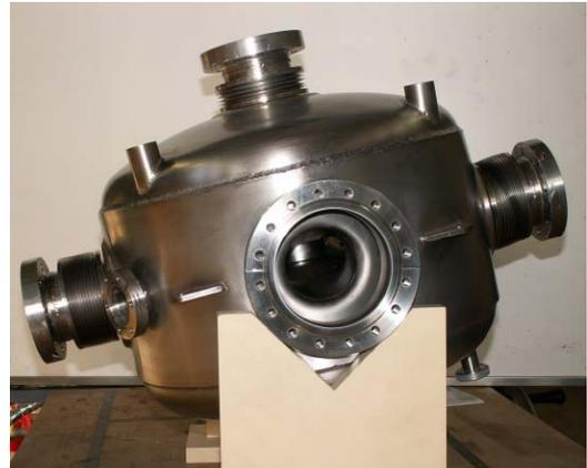
Figure 1:  $\beta$  0.15 spoke with its helium tank.
