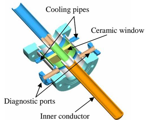
Figure 5: Power coupler for 2-gap spoke cavities.
