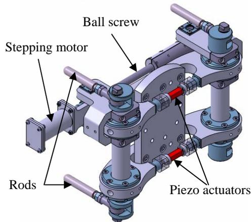
Figure 3: The cold tuning system for spoke cavities.
