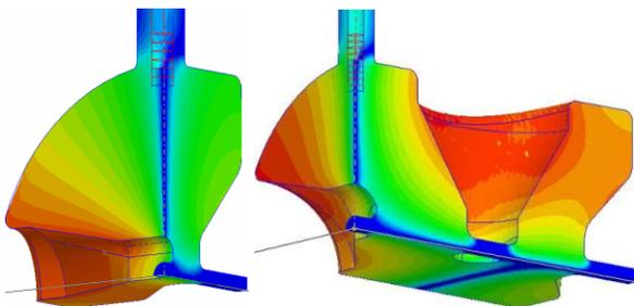
Figure 8. Magnetic field distribution in SSR1 and TSR with power couplers. The field strength increases from blue to green to yellow to red.
