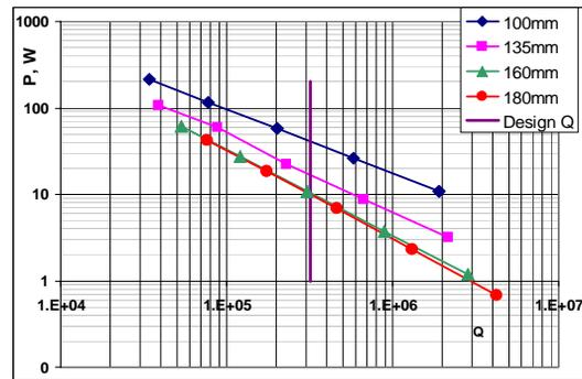
Figure 9. Pulsed power dissipation on the coupler tip vs. external Q of the coupler at different positions of the coupler.
