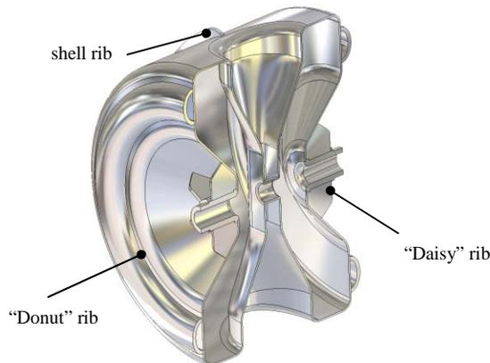
Figure 5. Cross section of the SSR1 structure. The stiffening ribs systems are highlighted.
