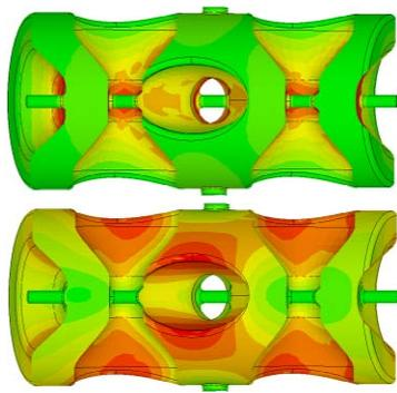
Figure 4. Surface electric (top) and magnetic (bottom) fields in TSR. The field strength increases as the color changes from green to yellow to red.
