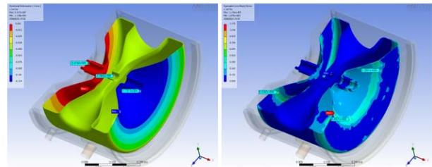
Figure 7 Left: longitudinal deformation [mm]; right: von Mises stress [10<sup>7</sup> Pa]. FEA boundary conditions: half structure studied (symmetry), He vessel fully constrained at fixed end wall flange (left in the pictures), 2000 N (~450 lbf) force applied at the inner end wall inside the bellows (right hand side). Max longitudinal deformation ~113micron, von Mises stress <12 MPa. Estimated frequency shift ~60KHz.
