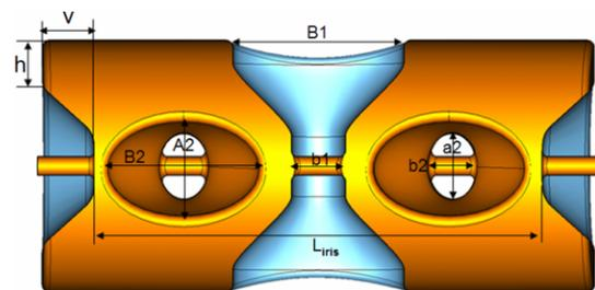
Figure 2. Cross section of the TSR with the main parameters used in the optimization process:  $L_{iris}$  – iris to iris length,  $a_1, b_1, A_1, B_1$  – ellipse half axis's of central spoke in base and axis area,  $a_2, b_2, A_2, B_2$  – ellipse half axis's of 1st and 3rd spokes in base and axis,  $h$  and  $v$  – end cup dimensions.
