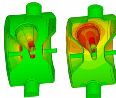
Figure 3. Surface electric (left) and magnetic (right) fields in SSR1. The field strength increases as the color changes from green to yellow to red.
