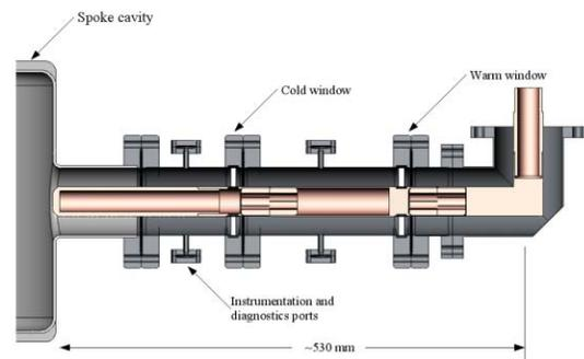
Figure 10. Mechanical design of the double window power coupler for the single spoke cavity.
