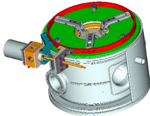
Figure 6. The slow tuner mechanism. One of the two He vessel shells is hidden with the purpose of showing the resonator. The slotted push/pull ring is shown in red. Each module has one slow tuner.
