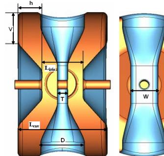
Figure 1. Cross section of the SSR1 and SSR2 with the main parameters used in the optimization process:  $L_{cav}$  – cavity length,  $L_{iris}$  – iris to iris length,  $D$  – spoke diameter,  $W$  – spoke width,  $T$  – spoke thickness,  $h$  and  $v$  – end cup dimensions.
