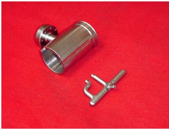
Figure 2: Modified HOM coupler configuration.
