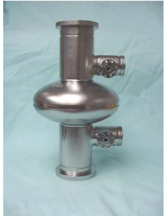
Figure 4: HOM Test Cavity.
