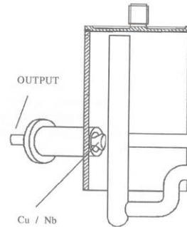
Figure 1: HOM coupler schematic (from Ref. [2]).
