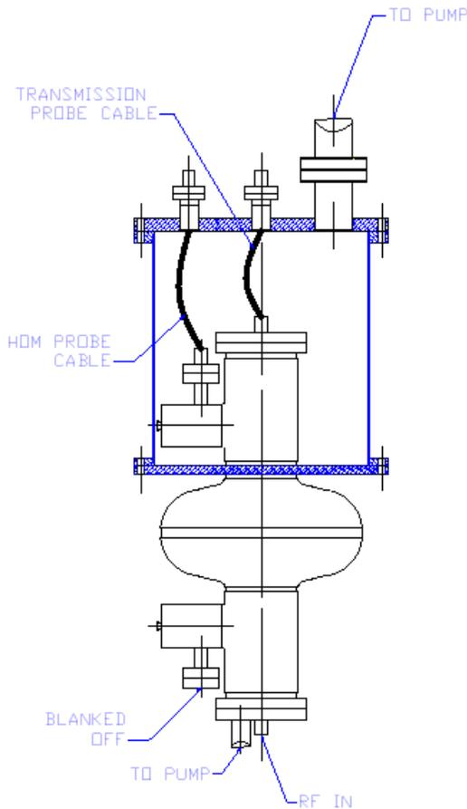
Figure 6: Schematic of isolated HOM coupler configuration.
