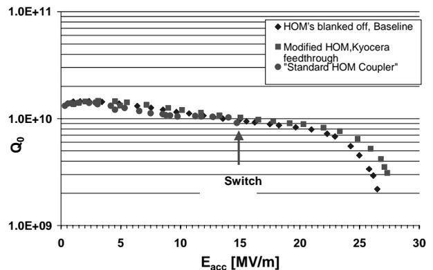
Figure 5: Comparison of the Q vs.  $E_{acc}$  performance of the test cavity with coupling probes attached to the “standard” (red circles) and “modified” HOM couplers (green squares). Included is a baseline test with both HOM couplers blanked off (blue diamonds).
