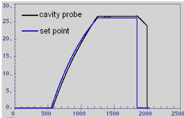
Figure 2: Amplitude plot obtained for a 600  $\mu\text{s}$  flat top at 27 MV/m.
