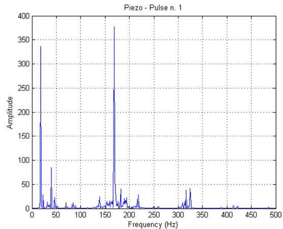
Figure 3: Background spectrum measurement with piezo.
