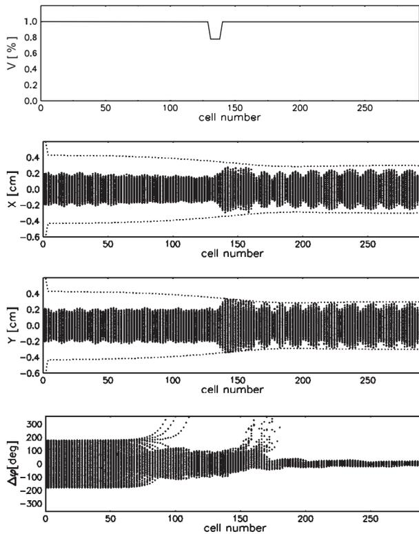
Figure 1: The effect of a perturbation in the electrode voltage distribution (first graph). In the middle of the structure, the voltage was reduced to 70% in defined range.
