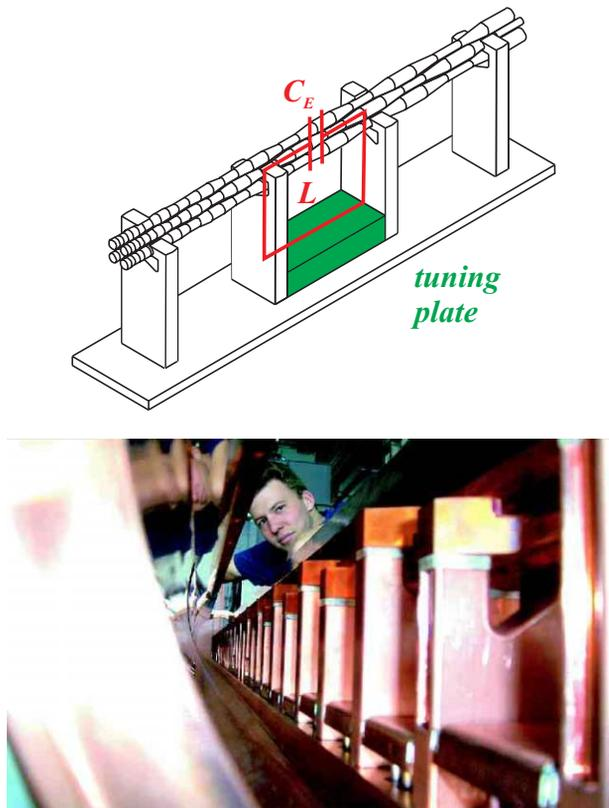
Figure 2: RFQ with 39 RF-cells and a tuning plate in each cell.
