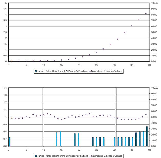
Figure 3: The electrode voltage distribution in the untuned, initial state and, below, the final tuning plate configuration with tuner plungers built in and high power coupling loop.
