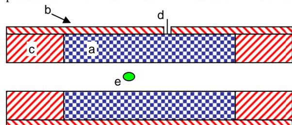
Figure 1: Longitudinal cross section of a typical dielectric loaded wakefield structure: (a) hollow dielectric cylinder; (b) copper waveguide; (c) copper end-piece; (d) coaxial antenna used as field probe; (e) electron bunch propagating along the axis of the structure.
