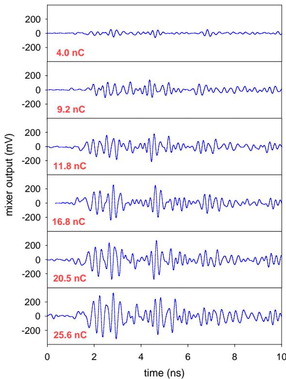
Figure 2: Output of RF mixer for various bunch charges that propagated through Structure 1.
