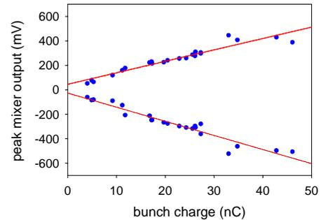
Figure 3: Peak values of the RF mixer output plotted as a function of the charge in the drive bunch.
