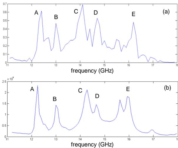
Figure 5: FFT of the radial component of the electric field (in arbitrary units), identifying the peaks A, B, C, D, E, respectively, as the modes  $HEM_{111}$ ,  $TM_{012}$ ,  $TM_{013}$ ,  $HEM_{112}$ ,  $TM_{014}$ : (a) measurement; (b) MAFIA simulation, taking into account the measured Q factor of each mode.
