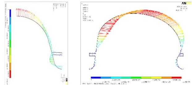
Figure 5: TeSLA and HR cell deformations caused by Lorentz force pressure (with stiffening rings).
