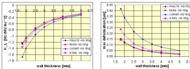
Figure 3: Mid-cell response to Lorentz force pressure (no stiffening rings).
