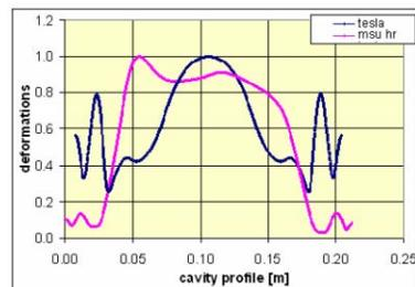
Figure 8: TeSLA and HR cell deformations caused by the Lorentz force along the cell profile (with stiffening rings).
