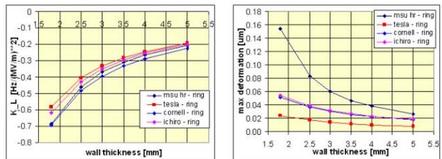
Figure 6: Mid-cell response to Lorentz force (with stiffening rings).
