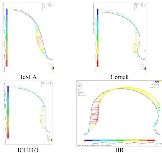
Figure 2: Cell deformations caused by the Lorentz force.
