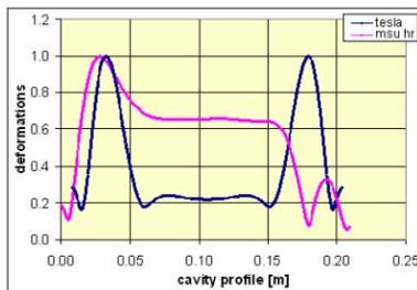
Figure 4: TeSLA and HR cell deformations caused by Lorentz force pressure along cell profile (no stiffening rings).
