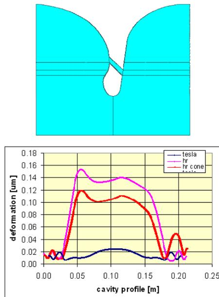
Figure 9: TeSLA and HR cell deformation caused by the Lorentz force along the cell profile (with stiffening rings and cone-shaped stiffening rings).
