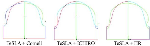
Figure 1: Mid-cell geometries.
