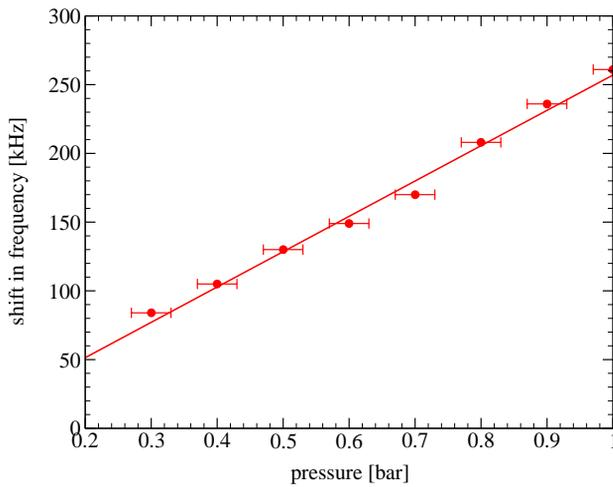
Figure 7: Shift in frequency due to change in external pressure.
