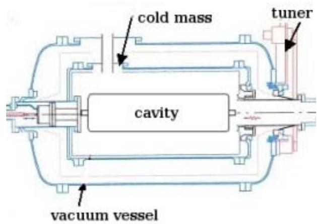
Figure 9: The horizontal cryostat with tuner and cavity.
