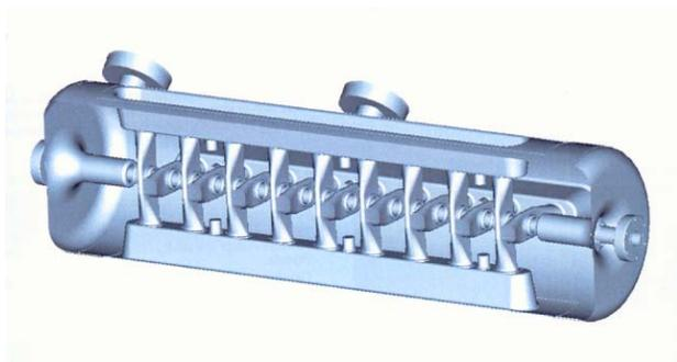
Figure 1: The 19-cell CH-prototype cavity.
