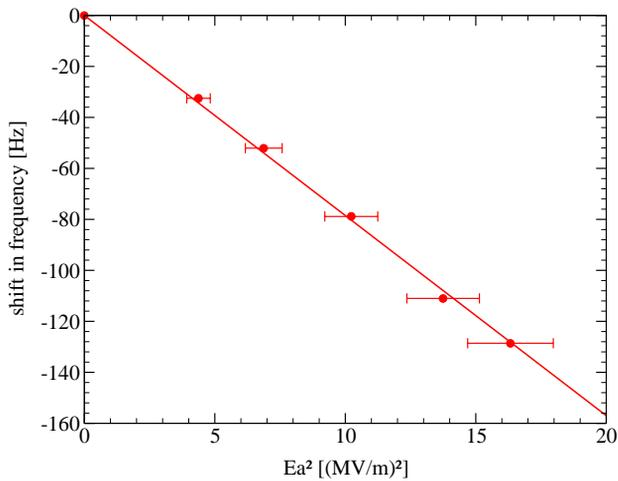
Figure 8: Shift in frequency due to change in electric field strength.
