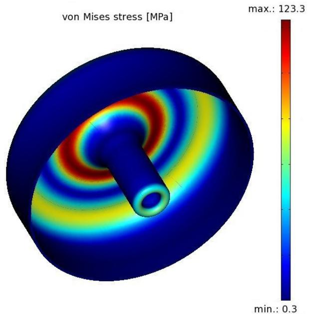
Figure 4: The deformed end cap from outside.
