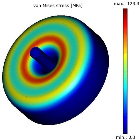
Figure 3: The deformed end cap from outside.
