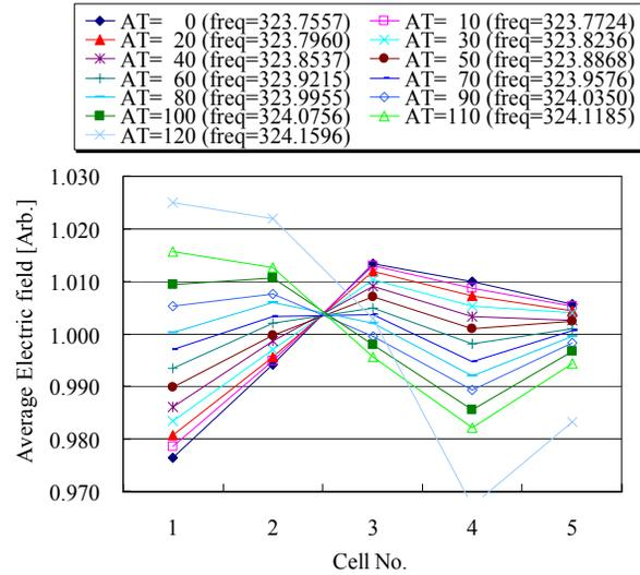
Figure 4: Average electric field at the various tuner length.
