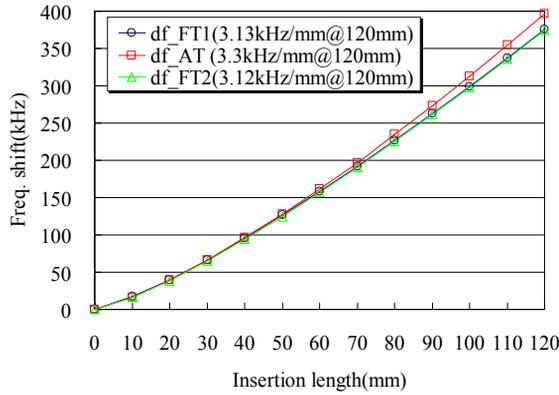
Figure 2: Insertion length of the tuner vs. Frequency shift.
