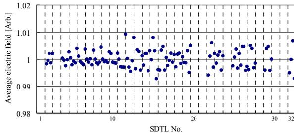
Figure 5: Adjusted electric field for all SDTL tanks.
