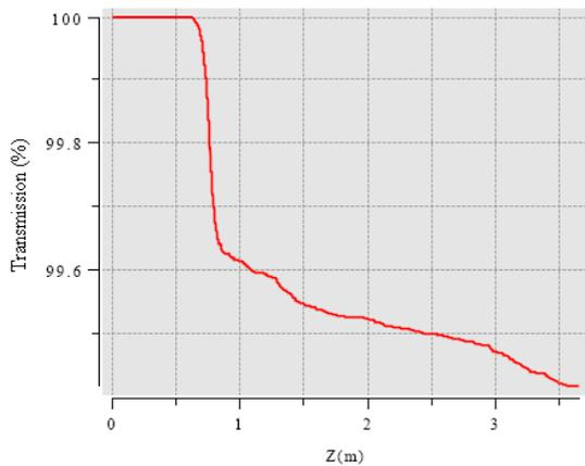
Figure 4: Beam Transmission versus RFQ length got by code TOUTATIS.
