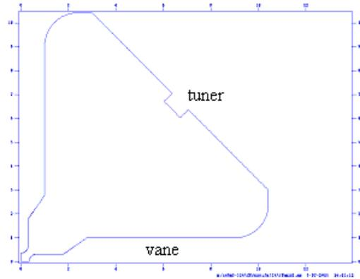
Figure 5: One quadrant of the RFQ transverse shape.
