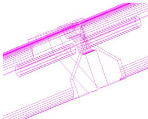
Figure 6: The simulated 3-dimension coupling cell.
