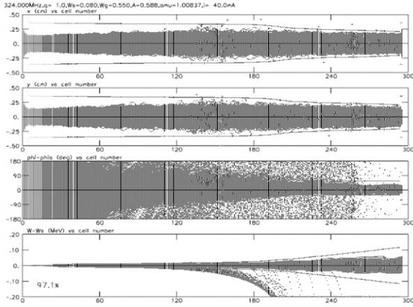
Figure 2: Beam dynamics in RFQ for a current of 40mA.
