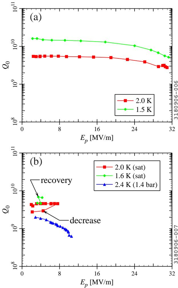
Figure 4. CW measurements with the cavity (a) under vacuum and (b) filled with liquid helium.
