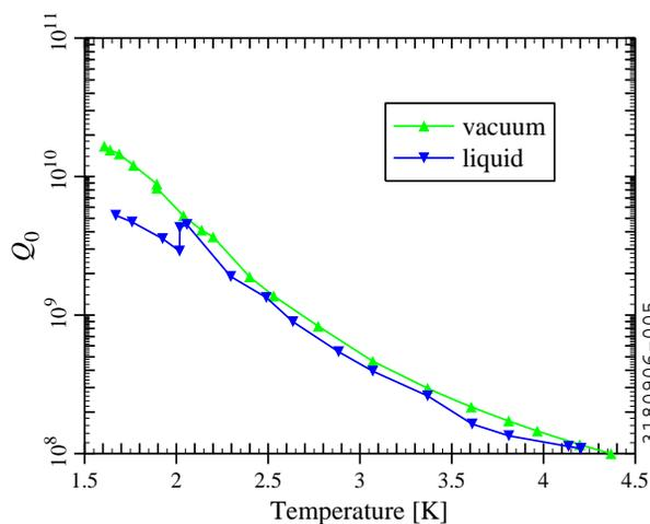
Figure 3. Comparison of the low-field  $Q$  between the cavity under vacuum and filled with liquid helium.
