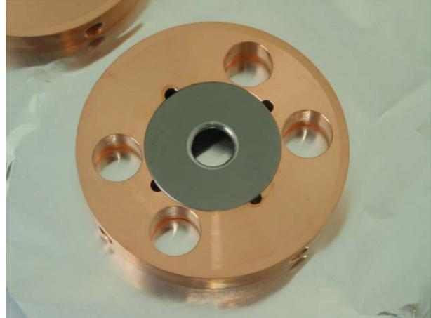
Figure 1: Tungsten-iris inserted into a copper disk forming together a cell of the rf structure. The beam aperture is 9.2 mm.
