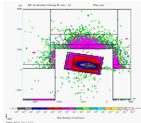
Figure 6: Mars calculation of the star density for the injection absorber.
