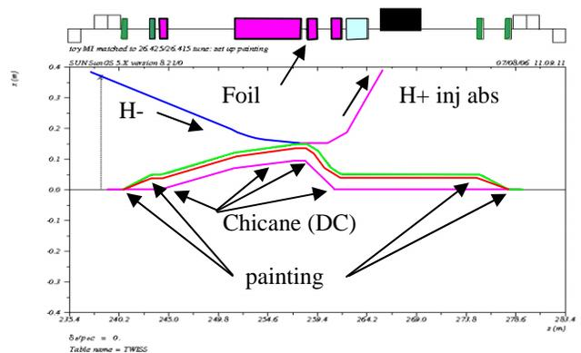
Figure 5: Layout of the injection straight section.
