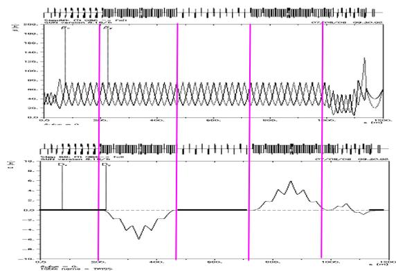
Figure 2: Lattice functions (top) and dispersion (bottom) of transfer line.
