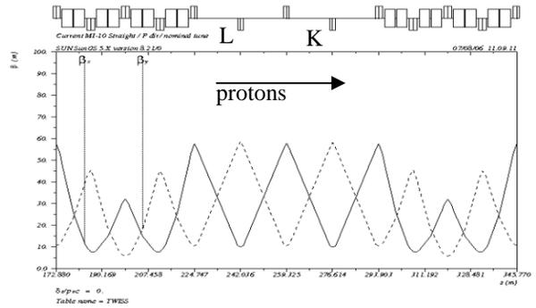
Figure 3: Current MI-10 injection straight section lattice functions.
