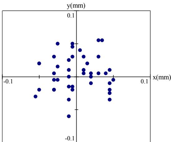
Figure 7: DT position of the DTL2 after the transportation.
