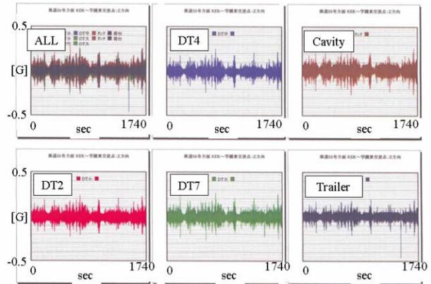
Figure 4: Acceleration data on the ordinary road.
