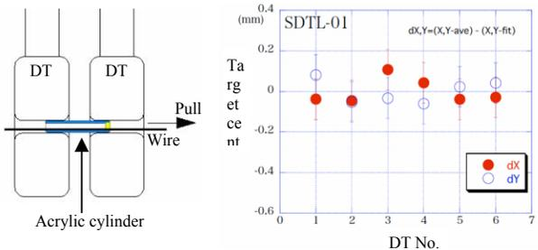
Figure 8: Schematic view of the measurement and the DT position of the SDTL1 after the transportation.
