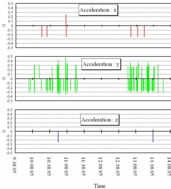
Figure 6: Acceleration data during the transportation.
