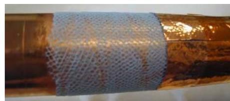
Figure 11: Polyethylene mesh as a spacer.
