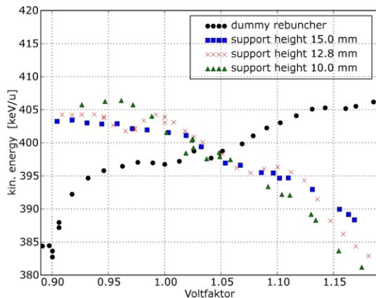
Figure 7: Specific energy in dependency of the voltage-factor for different mechanical rebuncher settings compared to the energy measurements with dummy rebuncher.
