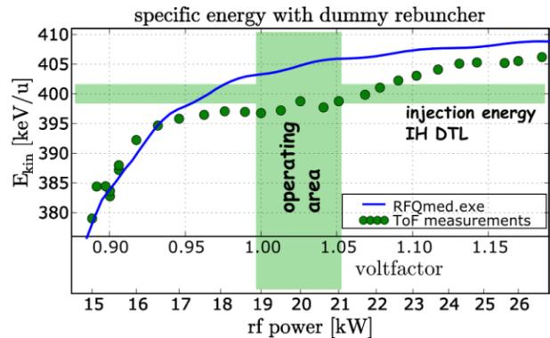
Figure 6: Comparison of simulated vs. measured beam energies at different RF power levels.
