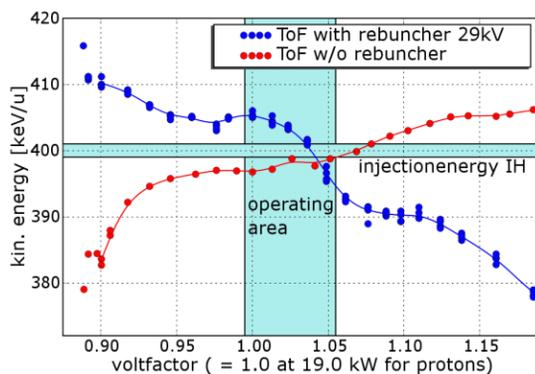
Figure 8: Estimated output energy of protons for the final mechanical rebuncher setting.
