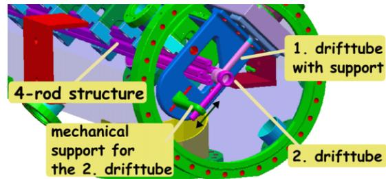
Figure 1: 3D-sketch of the integrated double gap rebuncher inside the RFQ tank.
