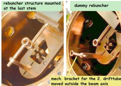
Figure 3: View on the installed rebuncher as well as on the drift tube tilted away from the beam axis but capacitively coupled to the tank wall (dummy rebuncher).
