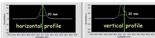
Figure 9: Horizontal and vertical beam profiles measured at the GSI testbench.
