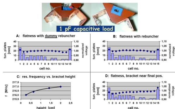
Figure 2: Photo of the utilized capacitive probe device. Height of tuning plates along the structure with estimated electrode field flatness without (A), with (B) rebuncher in its initial position. Adjustable range for the support holding (C). Flatness near final setting of the support (D).
