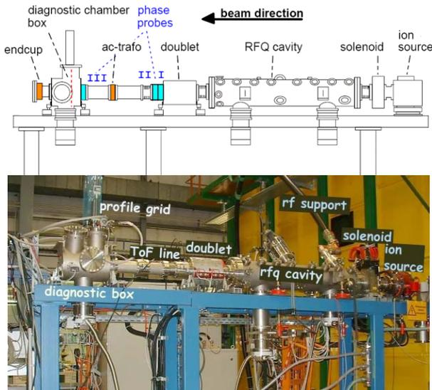
Figure 4: Layout and view of the testbench.
