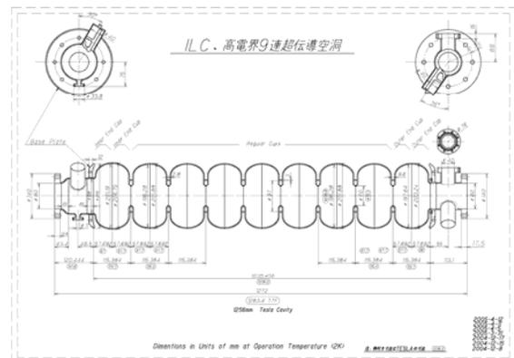
Figure 1: Draft of 9-cell ICHIRO high-gradient cavity.
