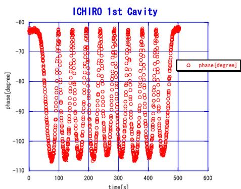
Figure 4: Field flatness of 1<sup>st</sup> ICHIRO cavity after pre-tuning. Pi-mode frequency is 1298.547 MHz.
