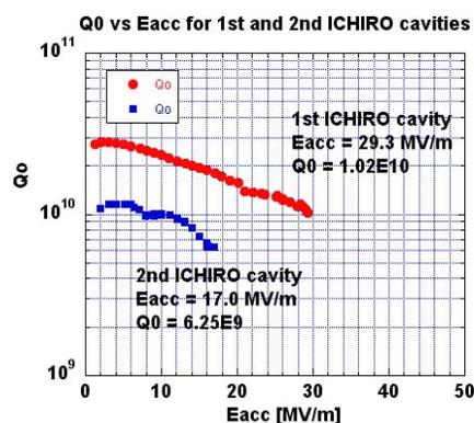
Figure 5: Vertical test results for 1<sup>st</sup> and 2<sup>nd</sup> ICHIRO cavities.
