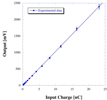
Figure 4: Linear relation of the input test charge to the output voltage. The input charge to the detection electronics is normalized by a beam charge.
