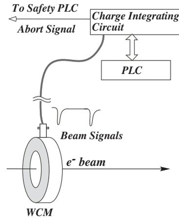
Figure 2: Block diagram of the beam-charge limit system using a wall-current monitor.
