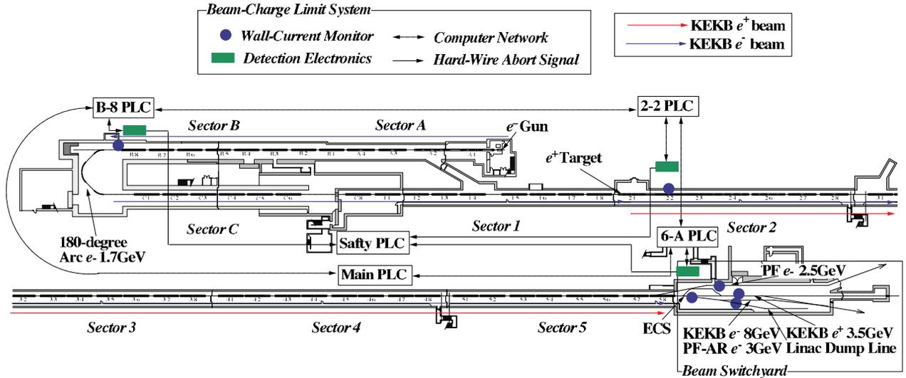
Figure 1: Locations of the beam-charge limit system for radiation safety at the KEKB injector linac.
