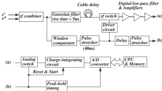
Figure 3: Block diagram of the detection electronics.
