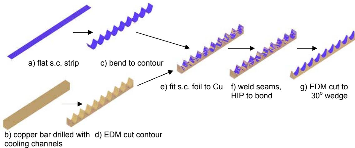
Figure 2: Fabrication sequence for constructing each wedge segment of a polyhedral cavity module.
