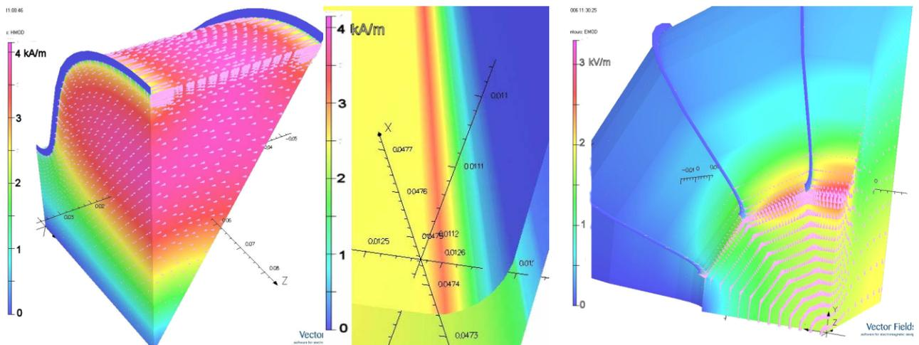
Figure 4: Field intensity distribution in the polyhedral cavity: a)  $\vec{H}$  in accelerating mode; b) detail of  $\vec{H}$  in slot in accelerating mode; c)  $\vec{E}$  in lowest-order deflecting mode.
