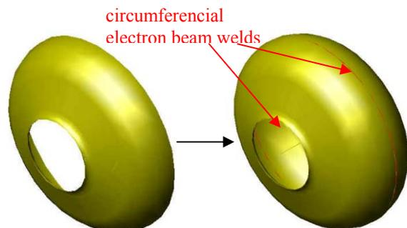
Figure 1: TESLA cavity cell construction.
