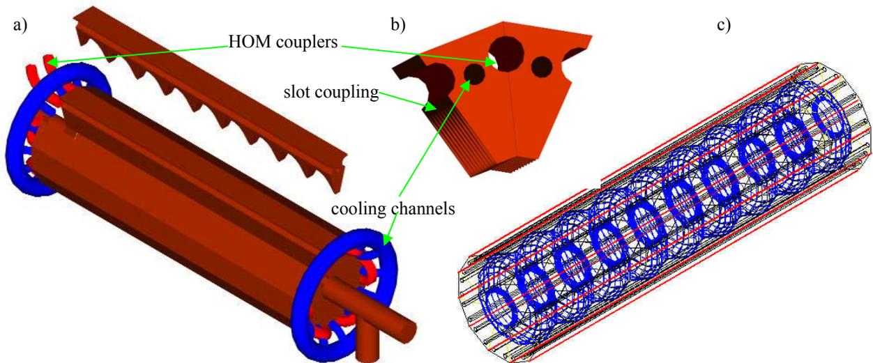
Figure 3: Assembly of 12 segments to make a polyhedral cavity module. a) polyhedral assembly, one segment withdrawn; b) detail of slot-coupled HOM waveguide and cooling channels; c) wire-frame showing interior cavity surface.
