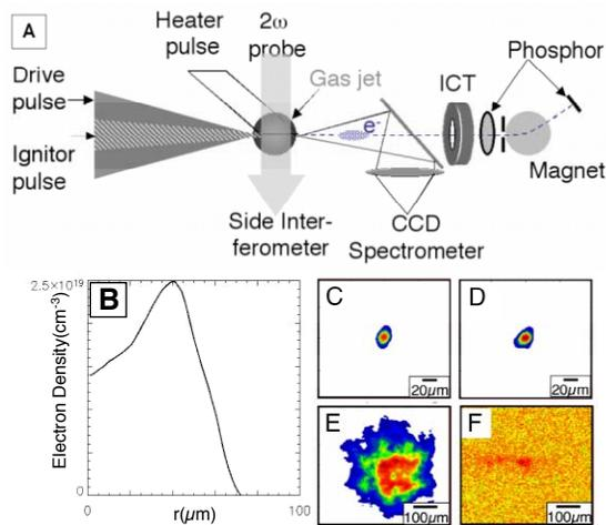
**Figure 1.** (A) Experimental setup showing the gas jet with laser beams and diagnostics. (B) The density profile of the channel obtained by Abel inversion of the side interferogram. (C-F) Mode images of laser propagation at 4 TW. The output image with the guide on (D) is indistinguishable from the input (C) indicating unaberrated propagation at twice  $P_{\text{crit}}$ . Unguided images show diffraction in vacuum (E) and ionization enhanced diffraction with the gas jet on (F).
