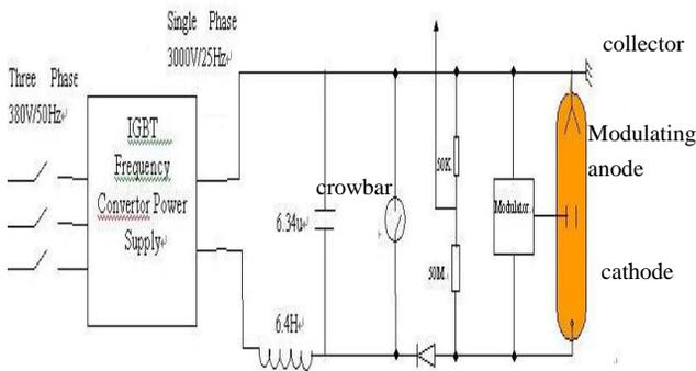
Figure 7: The proposed AC series resonance HV power supply for the klystron.
