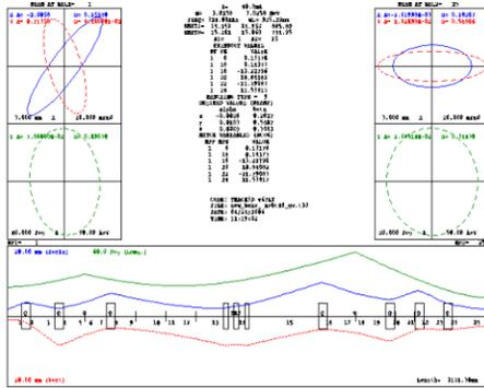
Figure 4: MEBT beam transport designed by TRACE3-D
