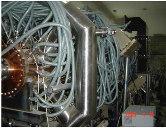
Figure 10: The ADS RFQ with a high-duty factor has been constructed at IHEP.
