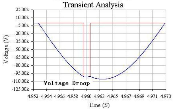
Figure 8: Flattop compensation by switching the DC pulse discharge at the moment a little before the bottom of sinusoid wave.
