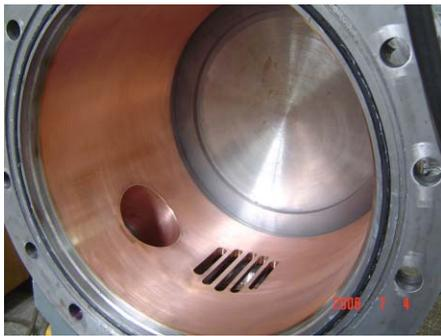
Figure 11: A steel-copper clad short test tank with all type of ports made with explosive clad technology.
