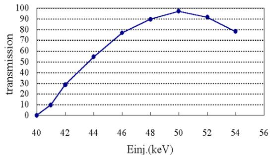
Figure3: RFQ transmission rate vs. injecting beam energy.
