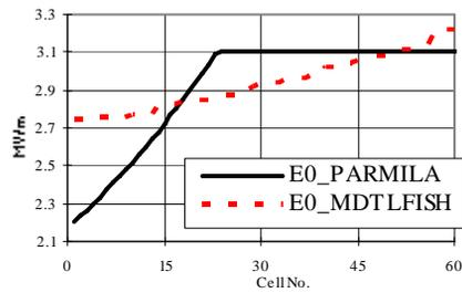
Figure 5: The solid curve shows the cavity design field input in PARMILA. The dashed curve shows the cavity field calculated by MDTFISH by using the cell data output from PARMILA.
