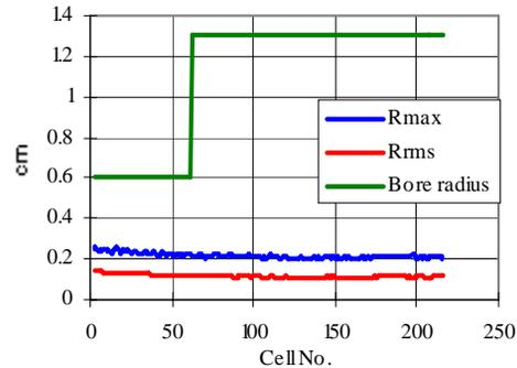
Figure 6: DT bore radius and rms/maximum beam radius along the DTL cell.
