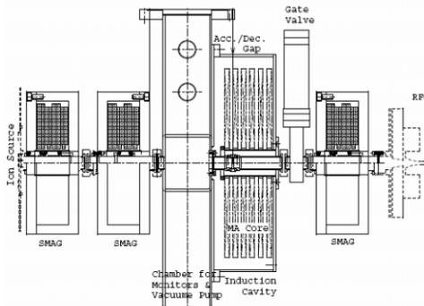
Figure 2: The LEBT with three solenoids and a magnet alloy loaded cavity for beam chopping.
