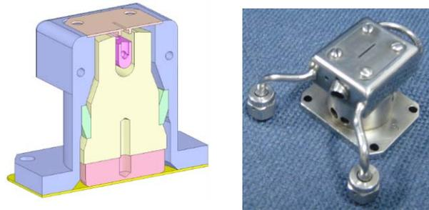
Figure 9: H<sup>-</sup> Pinning source body.
